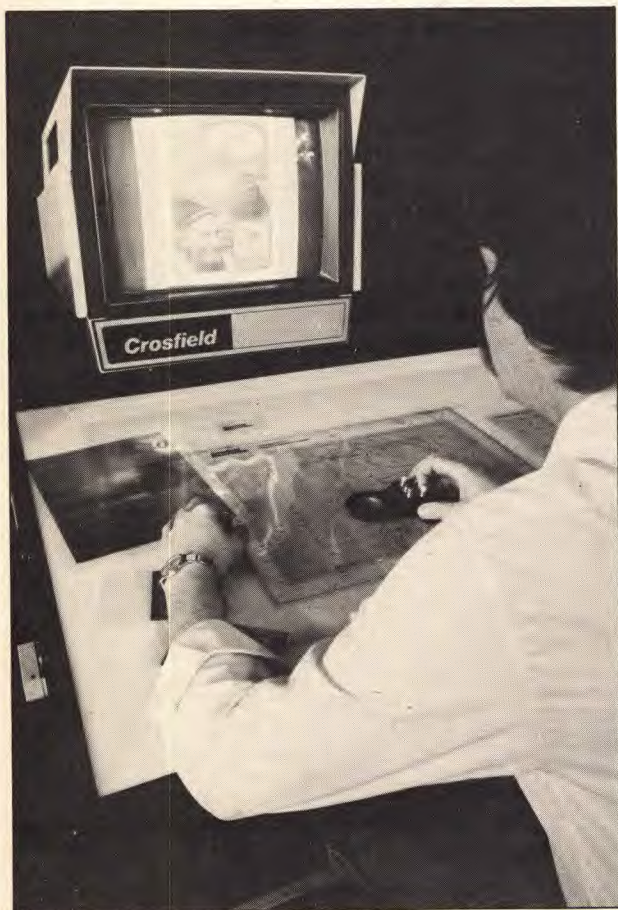
Crosfield Electronics: The operator at the planning table of the Magnascan 570 page composition system with new color monitor.
